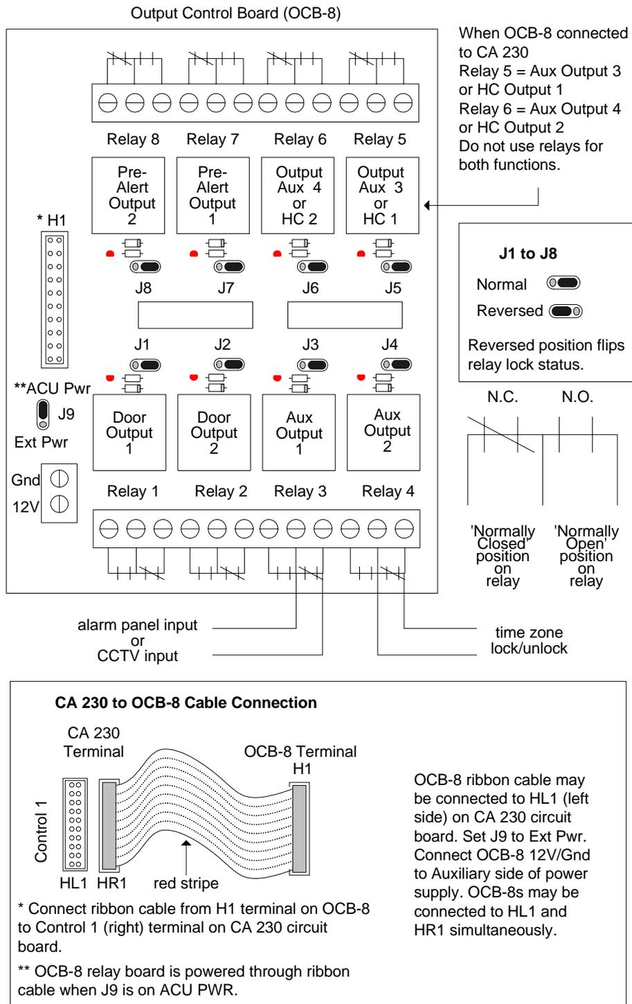
Figure 33 - Terminate Auxiliary Outputs CA 4300
