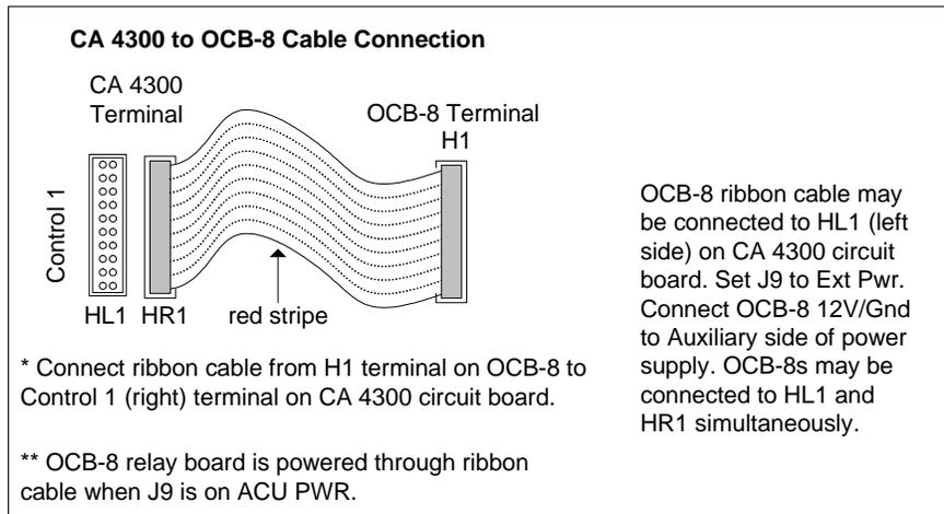
Figure 34 - Terminate Auxiliary Output CA 8300
