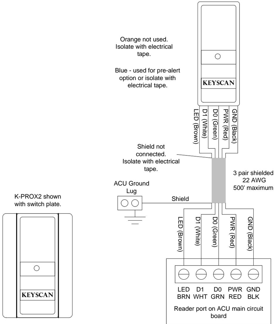
Figure 84 - Keyscan K-VAN Proximity Reader (125 KHz HID compatible)
