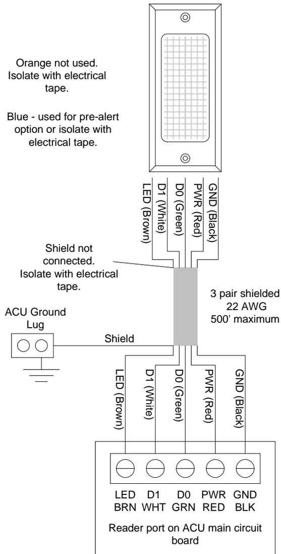
Figure 85 - Keyscan K-KPR Keypad / Proximity Reader (125 KHz HID compatible)
