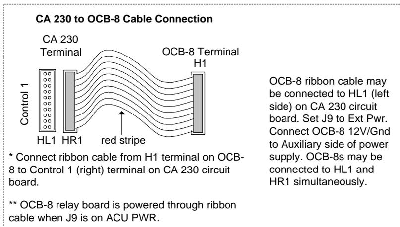
Figure 109 - Handicap Relay CA 4300/OCB-8 Connections
