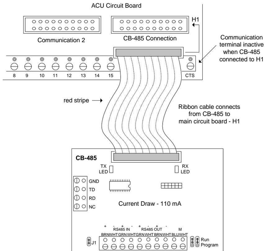
Figure 82 - CPB-10 Communication Test Points
