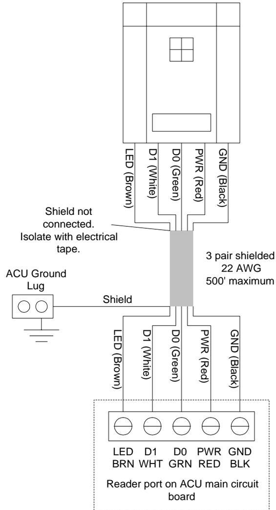
Figure 96 - Indala PX610 Wiring
