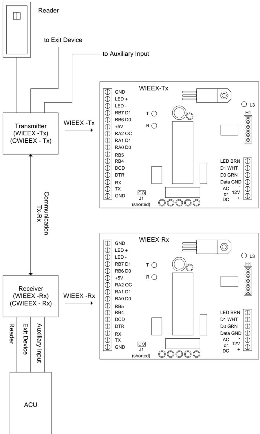
Figure 105 - WIEEX RS485 Transmitter/Receiver Connections
