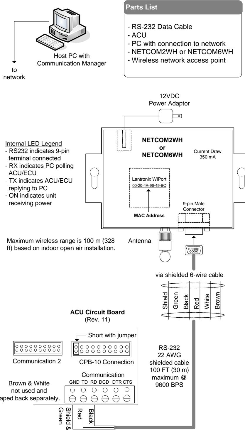
Figure 58 - Single ACU Communication - CB-485M/MC33H
