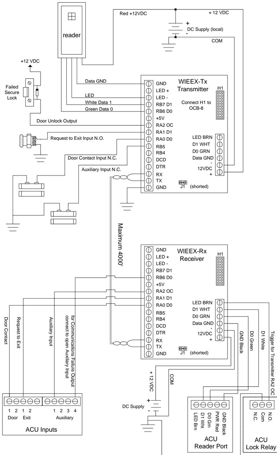
Figure 106 - CWIEEX - Coaxial Transmitter/Receiver Connections
