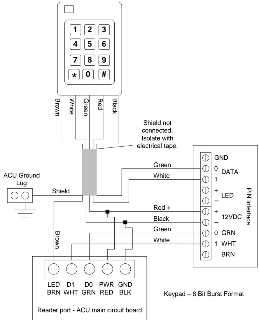
Figure 86 - HID-5395 Wiring
