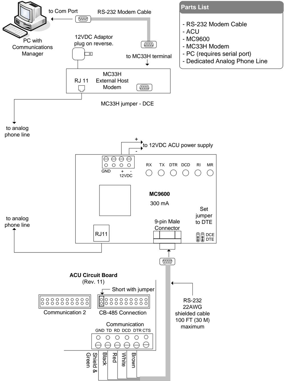
Figure 60 - Single ACU Communication - MC9600/MC33H/CPB-10
