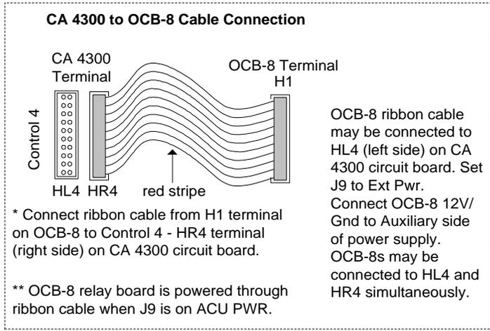
Figure 110 - Handicap Relay CA 8300/OCB-8 Connections
