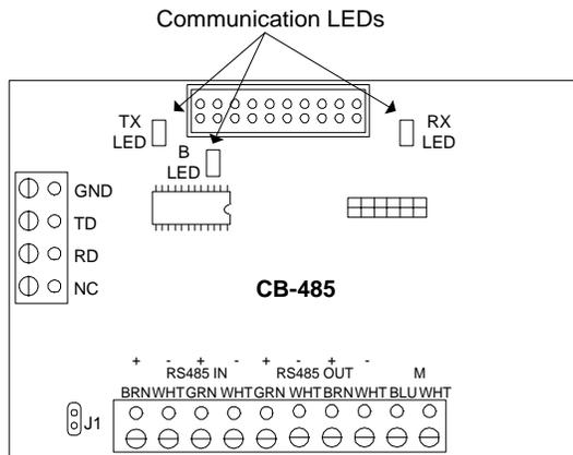
Figure 77 - Communication LEDs on CPB-10
