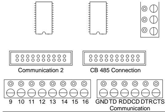
Figure 81 - CB-485 Communication Test Points
