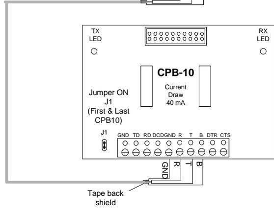
Figure 67 - Multiple ACU Communication - NETCOM2 or NETCOM6/CPB-10
