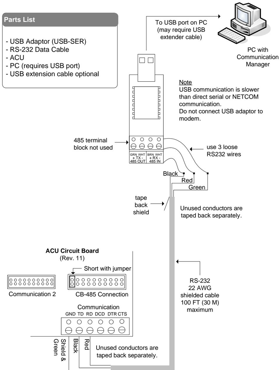
Figure 48 - Single ACU Communication - USB Adaptor/CB-485 (RS232)
