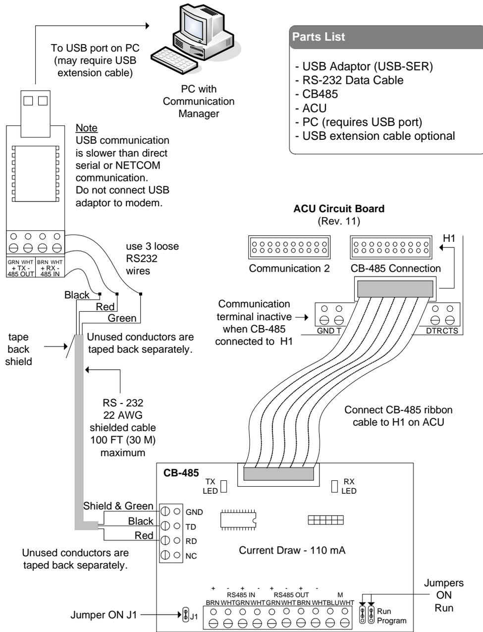
Figure 50 - Single ACU Communication - USB Adaptor/CPB-10 (RS232)
