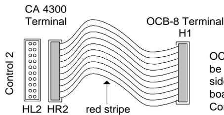
\* Connect ribbon cable from H1 terminal on OCB-8 to Control 2 - HR2 (right) terminal on CA 4300 circuit board.
