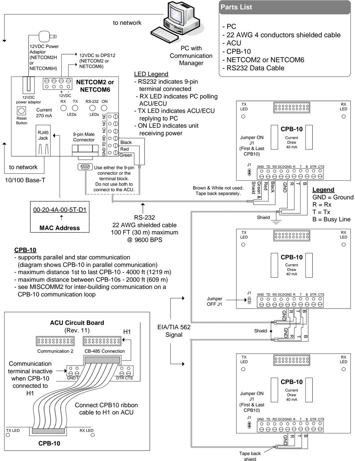
Figure 68 - Multiple ACU Communication - NETCOM2P or NETCOM6P/CB-485 (1 to 1)
