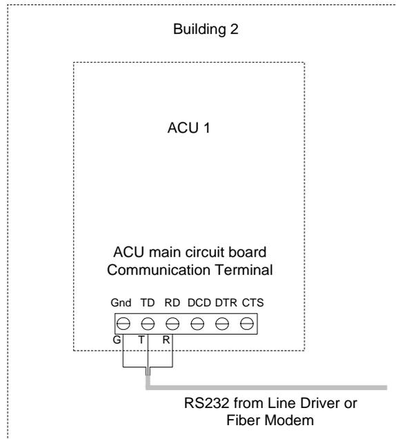
Figure 116 - MISCOMM2 Inter Building Communication to Multiple ACUs
