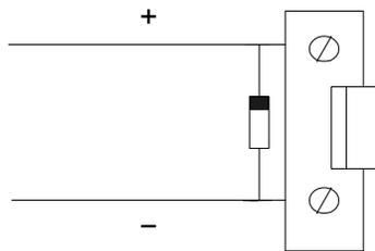
Figure 15 - Typical Door Maglock Connection
