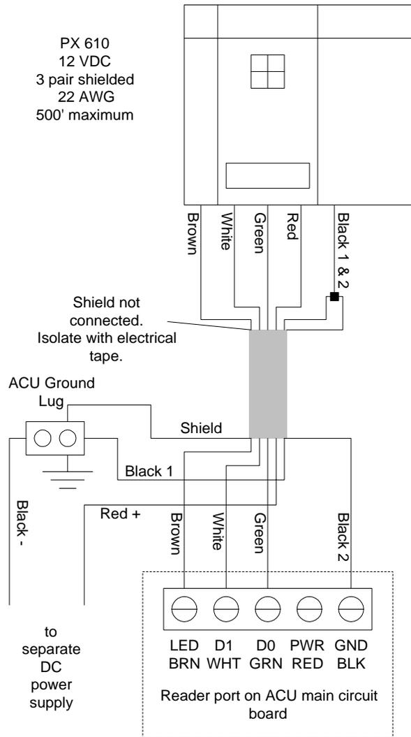
Figure 97 – Indala PX 620 Wiring
