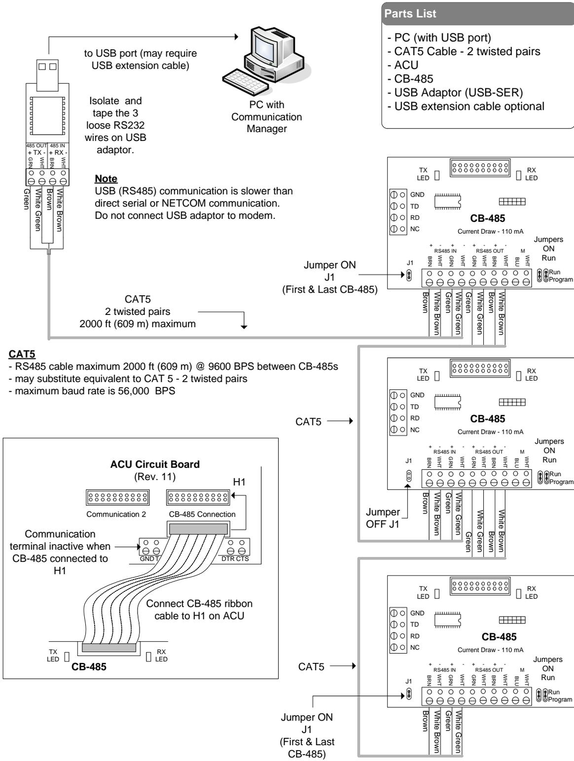
Figure 65 - Multiple ACU Communication - USB Adaptor/CPB-10
