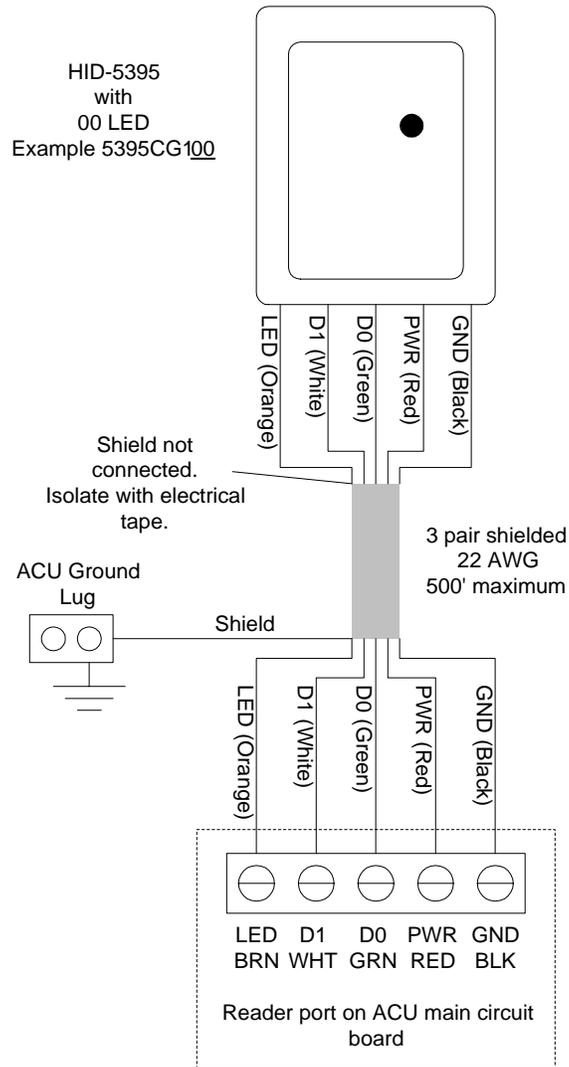
Figure 87 - HID 5365 / 6005 Wiring
