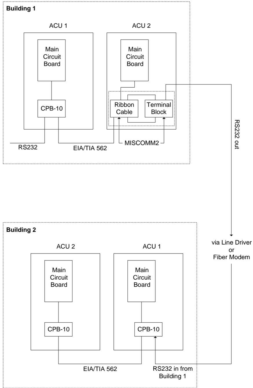
Figure 117 - MISCOMM2 Connections to Multiple ACUs
