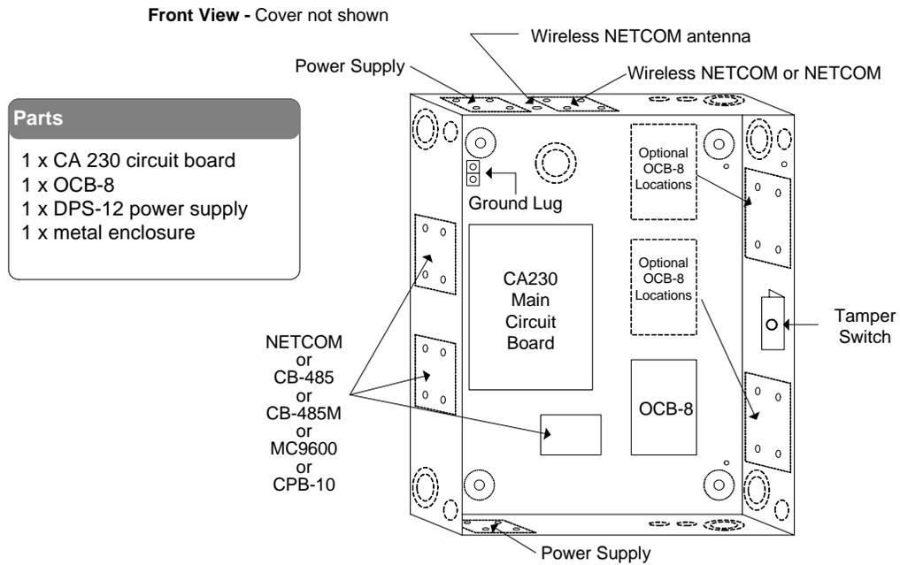
**Figure 7 - CA 4000 with Circuit Board Mounting Positions**
