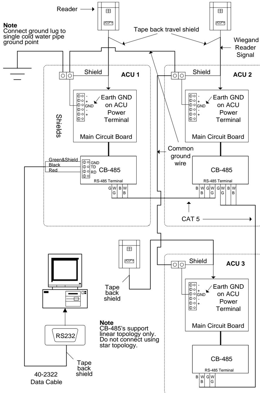
Figure 2 - Grounding Access Control Units and Cables with CPB-10s
