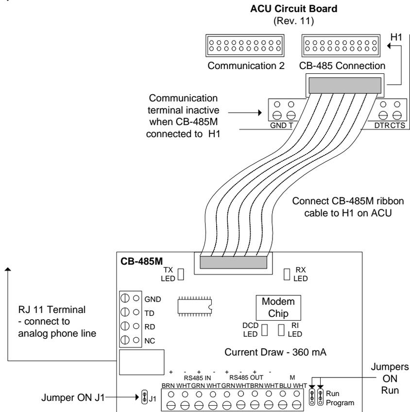
Figure 59 - Single ACU Communication - MC9600/MC33H
