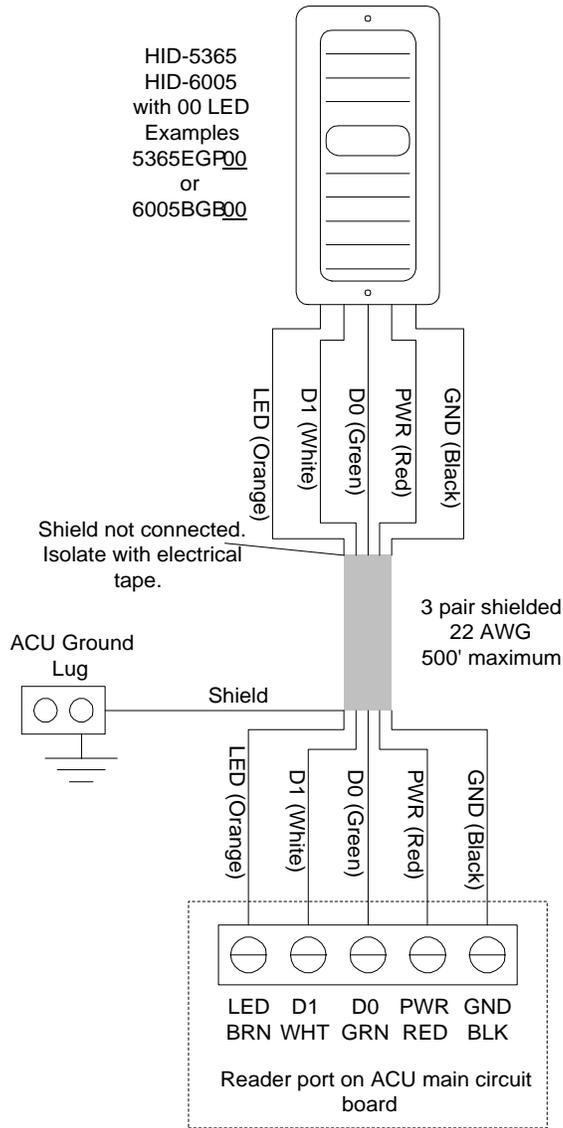
Figure 88 - HID 5355 Wiring
