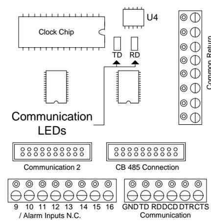
Figure 76 - Communication LEDs on CB-485
