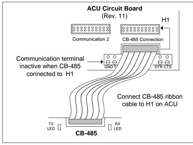
Figure 69 - Multiple ACU Communication - NETCOM2 or NETCOM6 (1 per ACU)
